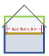
RR Type 2 has an accessible vertical continuation of the external wall of the storey below which is **less than 1.8 m** for at least 50% of the common wall (excluding gable ends or party walls).
