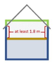
Similar to RR Type 2 but where the accessible vertical continuation of the external wall of the storey below is **1.8 m or more** for at least 50% of the common wall (excluding gable ends or party walls). This is NOT a Room in Roof and must simply be treated as a separate storey.
